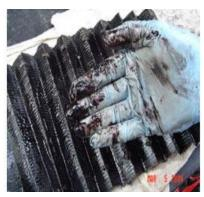
**Filter plugging can have several causes**. For example, **low temperatures can cause wax crystallization**, which can lead to filter plugging. An example would be using summer diesel in cold weather. Wax or paraffin is part of the diesel fuel. An additive such as a Winter Fuel Catalyst with Anti Gel is the answer to that problem.
