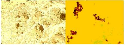
The solids that form as the result of the inherent instability of the fuel and the natural process of degradation will accumulate in the bottom of your tank. The sludge will form a coating or bio-film on the walls and baffles of the tank, plug your filters and impact combustion efficiency. Eventually it will clog fuel lines and ruin your equipment.
