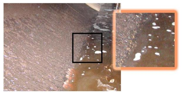
Temperature, humidity and condensation are very important factors in managing fuel integrity. The presence of free water provides the medium for microbiological growth that results in the formation of slime and acids causing corrosion of metal surfaces such as storage tanks, pumps, injectors, etc.
